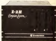
Model Z-2H 11 Megabytes of hard disk storage. Up to 512 KiloBytes of RAM/ROM 780 KiloBytes of floppy disk storage.
